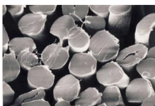
Each cotton fiber is swollen and has a round cross section.
